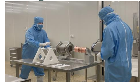
RFD PIM assembly in clean room designed by R.Leuxe & L.Giordanino (CERN)
