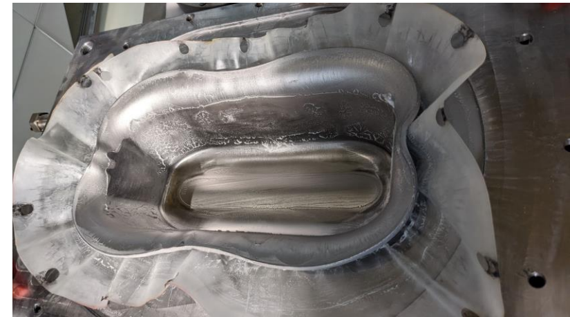
Preparation of the RFD Pole forming trials held at CERN Main Workshop (May 2022).
