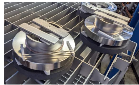
Brazed assemblies preparation, with Nb RRR witness samples. By F. Motschmann.
