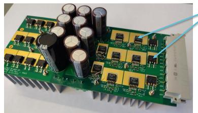
Innovative through-PCB cooling of semiconductors!
