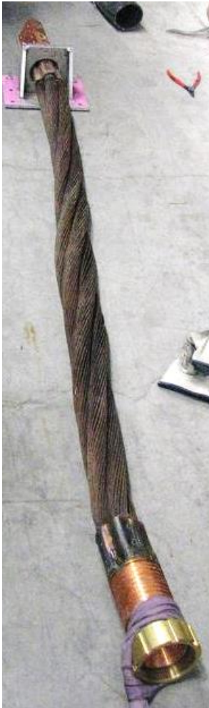
CABLE BUNDLE CRIMPED ON THE LUG: WCC WITHOUT SPRING (2000 mm 2 )
