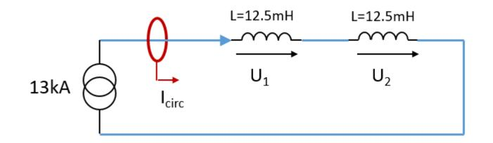
di/dt max: 12 A/s Uind<sub>max</sub>: 150 mV
