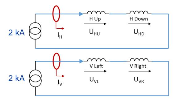
di/dt<sub>max</sub>: 15 A/s Lcircuit: 58mH .. 232 mH Uind<sub>max</sub>: 870 .. 3480 mV
