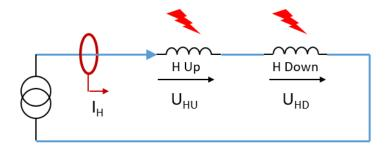
$U_{quench} = U_{HU} - U_{HD} \rightarrow$  insensitive to quench voltage if present on both coils
