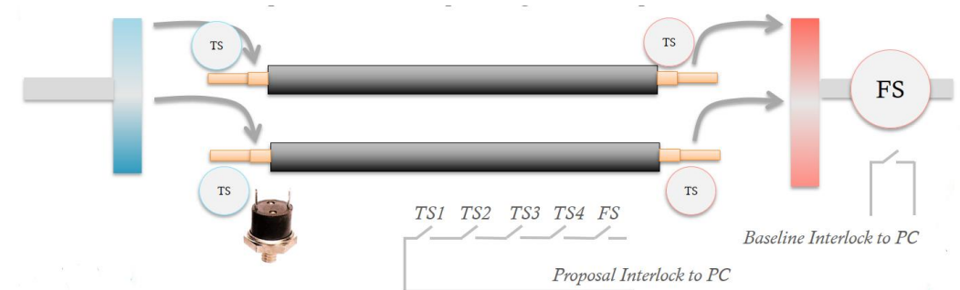
Interlock redundancy elements, courtesy of S. Yammine
