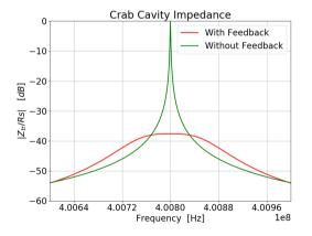
Closed Loop cavity impedance
