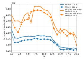
B1, positive oct. polarity,  $\tau_b = 1.2$  ns, Nb=2.3e+11 , M=3564 , damp=0.1
