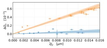
Effectively loose 20 % of available LHCB1 MO strength at  $30\,\mathrm{cm}$  due to residual  $b_4$
