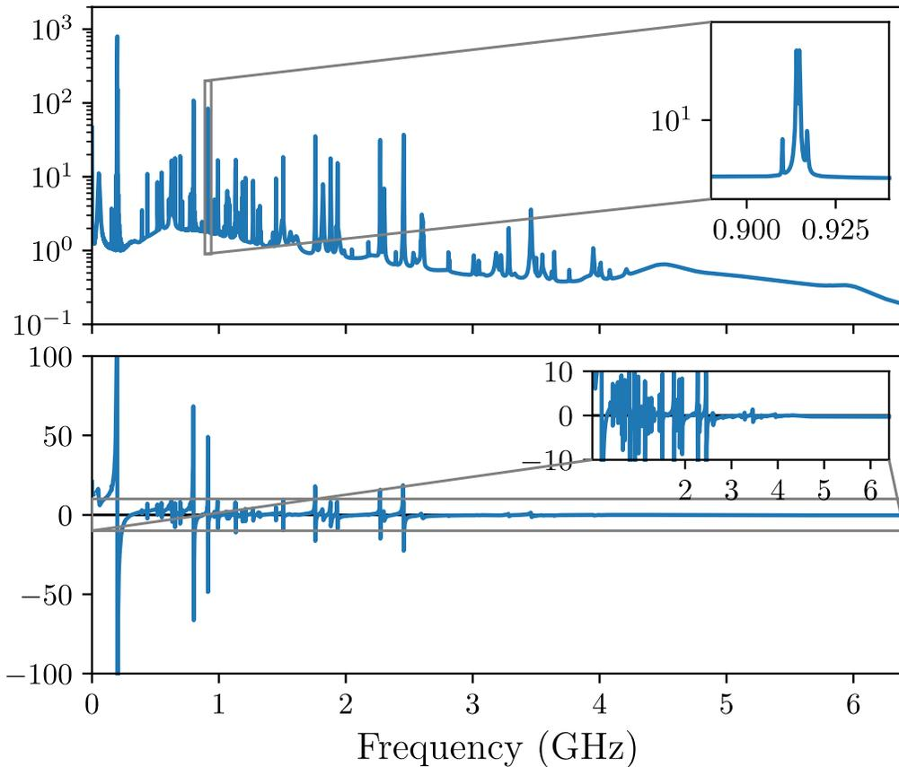
Coupled-bunch instability in **SPS** uniform filling with 25 ns spacing,  $V_{\text{rf}} = 7.2$  MV,  $E = 450$  GeV (MELODY)
