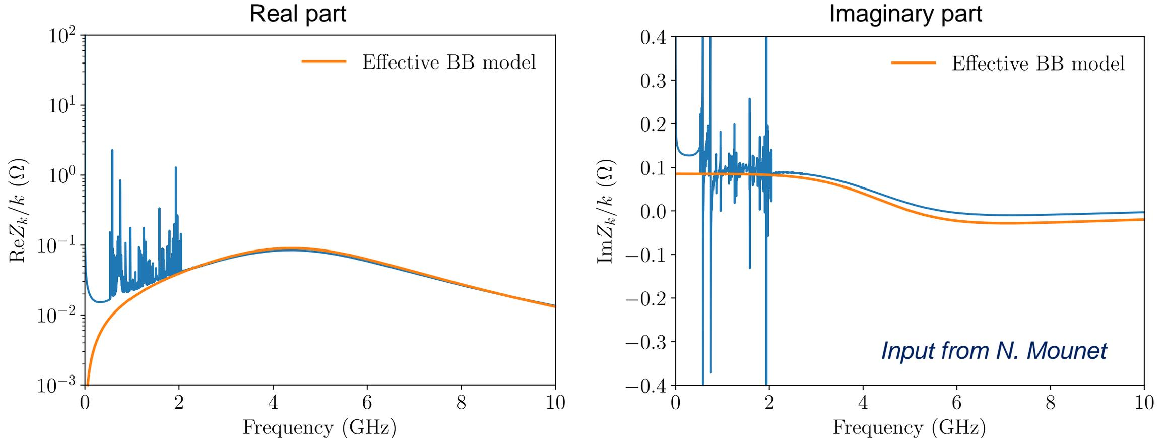
BB contributions from different elements are added as a single BB resonator with  $f_r = 5$  GHz
