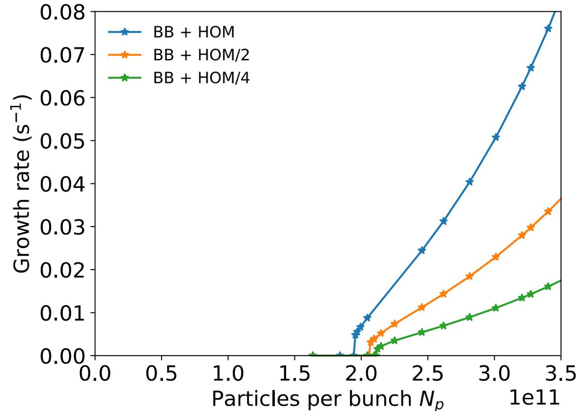
$$E = 450 \text{ GeV}, V_{\text{rf}} = 8 \text{ MV}, \mu = 2, \tau_{4\sigma} \approx 1.2 \text{ ns}$$
