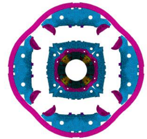
Stress during bladder operations, Symmetric loading, bladder slots + cooling holes
