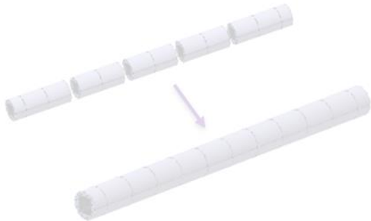
Assembly of the yoke-shell structure
