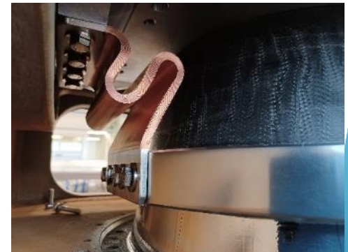
Support post thermalization strap installed
