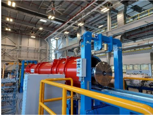
Dummy cold mass in vacuum vessel
