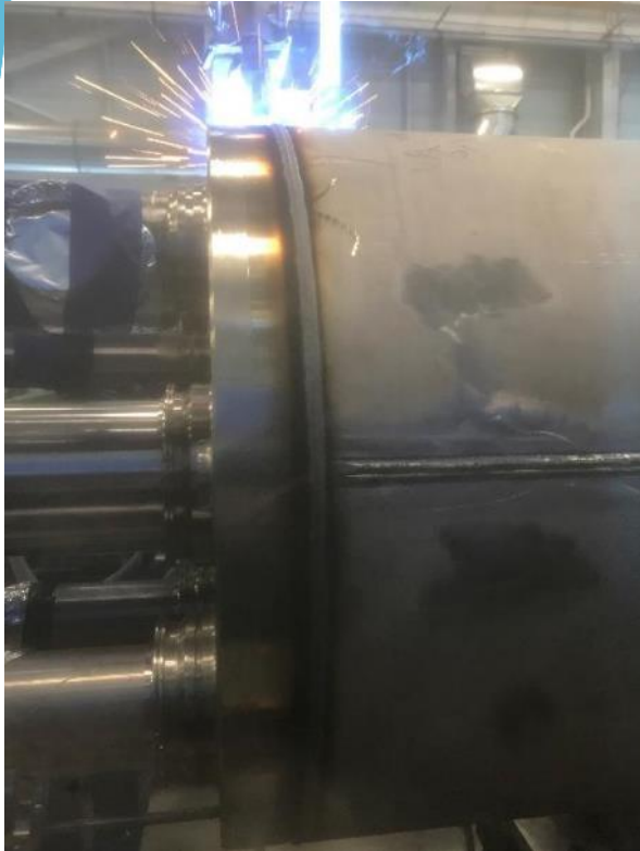
End Cover Welding
