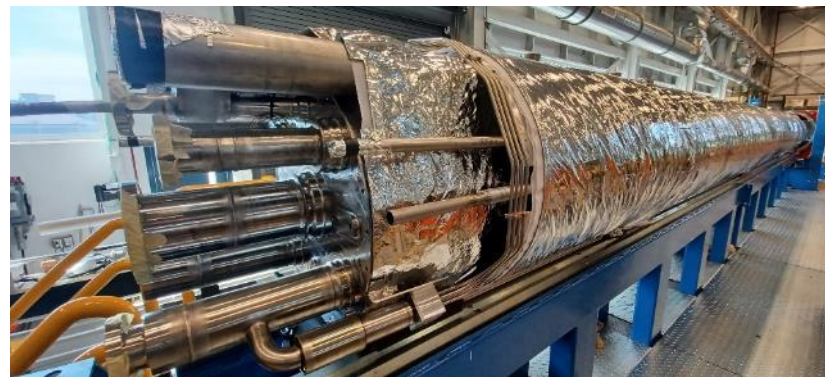
Cold mass and thermal shield integrated and insulated
