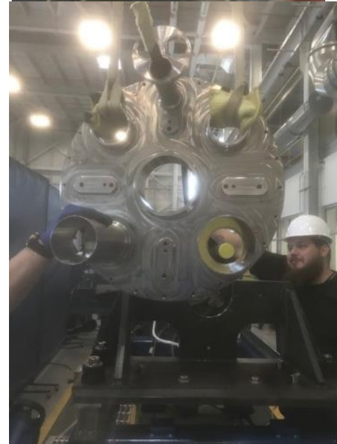
End Cover aligned and tacked
