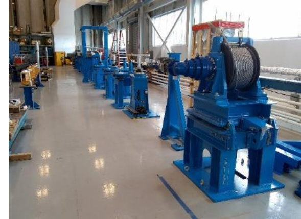
Cryostatting winch and vessel supports
