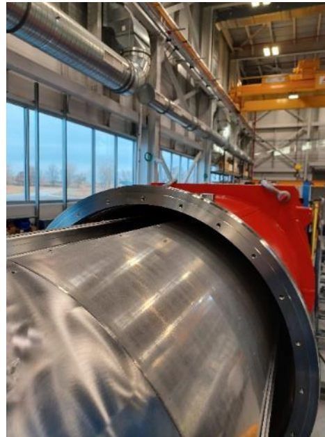
Dummy cold mass and thermal shield being inserted into vacuum vessel
