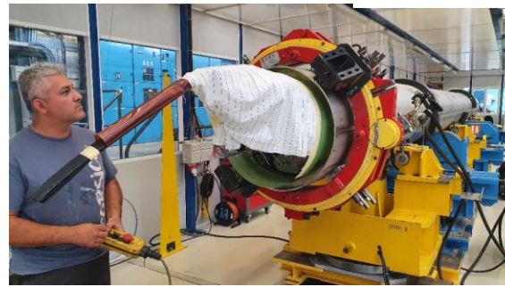
Shell extremity cutting and welding preparation machining for the end covers
