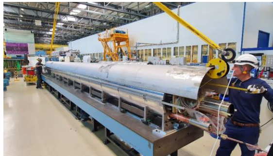
Shell installation and alignment
