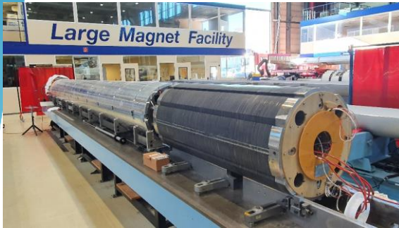
Quad. and corr. Alignment on the assembly bench
