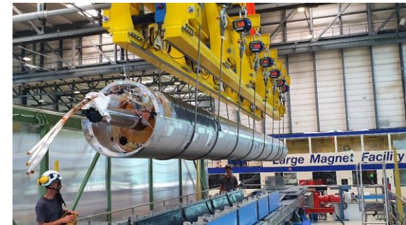
Transfer to the welding press conveyor
