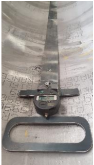
Developed length measurement tool and calibration checks
