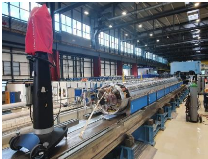
Magnet yoke measurements with the laser tracker
