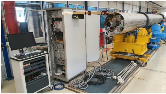
Mag. measurement to orient the field to gravity Welding of the supports
