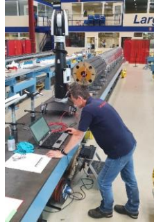
Magnet yoke measurements with the laser tracker
