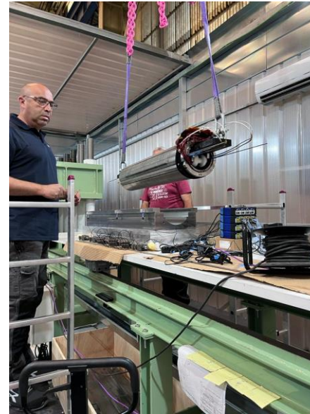
Inner dipole entering the collaring press
