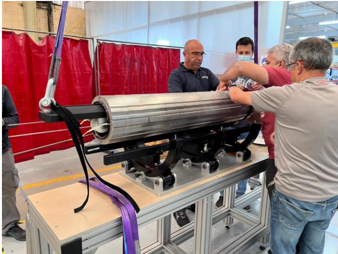
Inner dipole ready for collaring press
