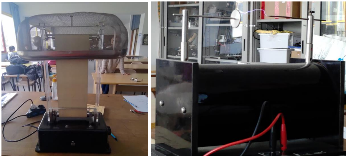
Fig. 1. Testing a Van der Graaf Generator on the left and a Ruhmkorff coil on the right.
