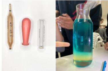
Fig. 1. Experiment performed in a school. On the left typical objects used as divers; on the right the jar filled with coloured density-stratified liquid with a diver in equilibrium at a given height
