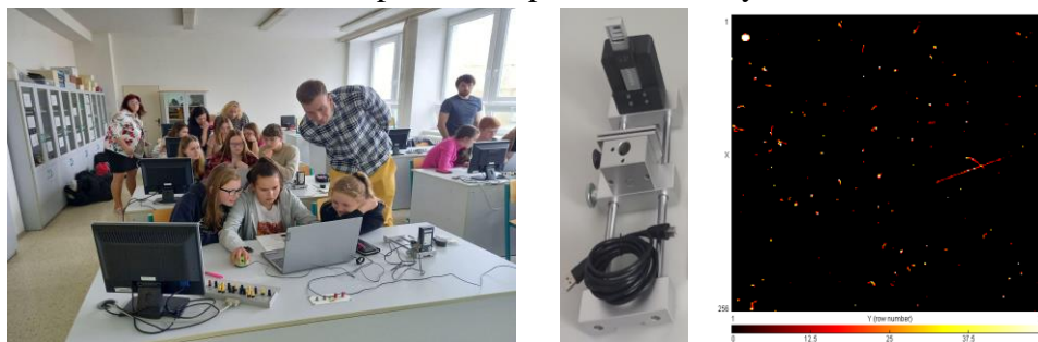
Fig.1. Left - Elementary school students performing observations at classes, Centre - Detail look at the set-up of the particle camera instrument, Right - observation performed with a bare detector without any radioactive sample placed close to the detector showing non-zero activity proving presence of background radiation.
