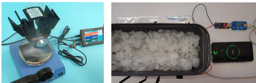
Fig. 1. Fireplace fan and mobile phone charger with Peltier cell.
