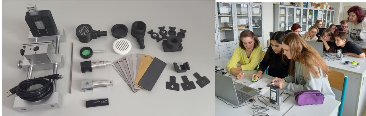
Fig. 1. Left - SESTRA kit (School Education Set with Timepix for Radiation Analysis) accessories deployed on the table (namely: MiniPIX EDU particle camera, mounting rails, camera holder, radiation source holder, uranium glass, thoria rod, Am241 300 kBq gamma source, Am241 9.6 kBq alpha/gamma source, container with potassium salt, empty container for samples, set of shielding plates, radiography adapters heads, sample patterns for alpha radiography and gamma radiography, vacuum cleaner grate adapter, USB cable, USB flash drive with control and visualisation software); Right - Elementary school students at classes observing properties of alpha particles under supervision of a physics teacher..
