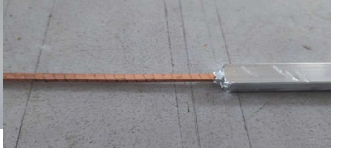
Short Al-stabilized ReBCO Stacked tape cable
