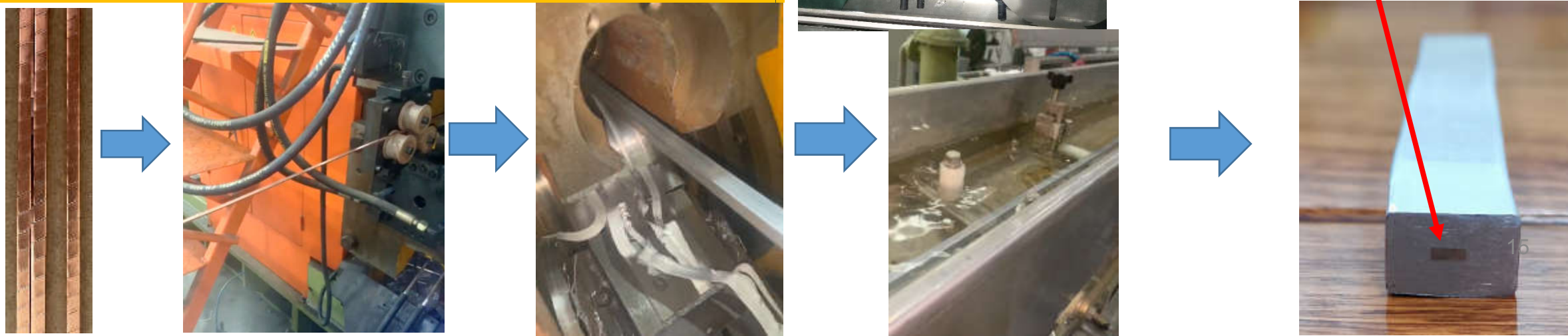
The process of Al-stabilized ReBCO Stacked tape cable
