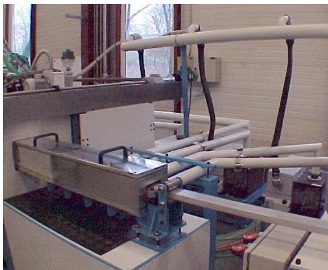
Entrance Air-Vacuum lock
