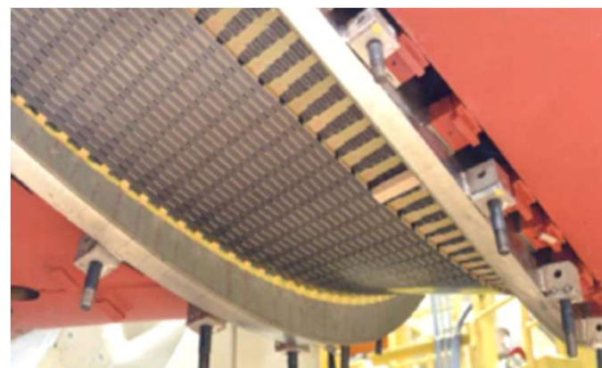
On-site Winding (450 turns x 2 coils)
