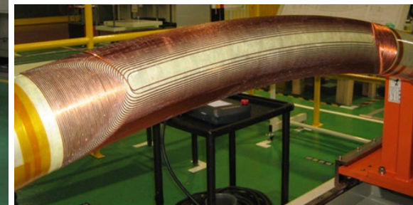
Saddle-shaped and curved coil manufactured by 3D winding technology
