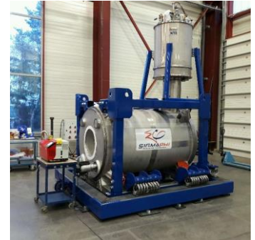
Quad for JLAB (16T/m, 4m)
