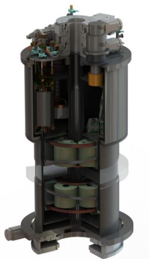
Quad for JLAB (16T/m, 4m)
