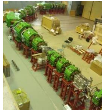
ACCULINA (JINR) 70m heavy ion beamline
