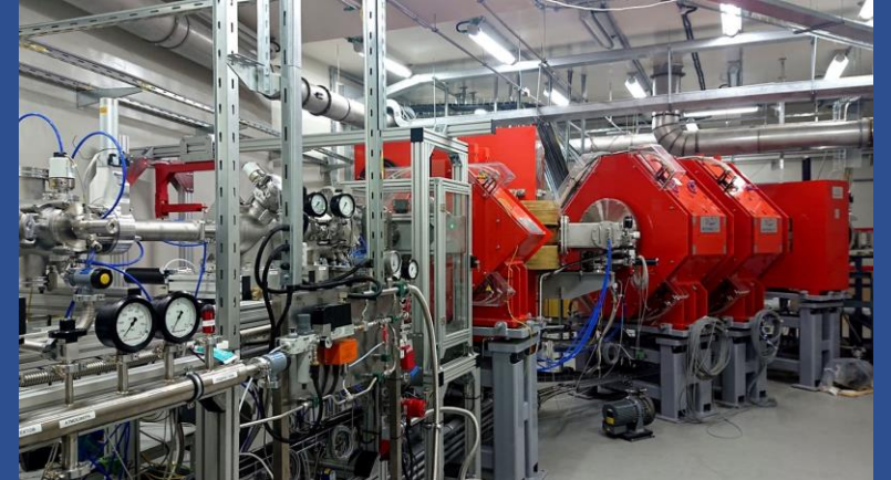
JINR (Russia) He gas filled separator GFS-II
