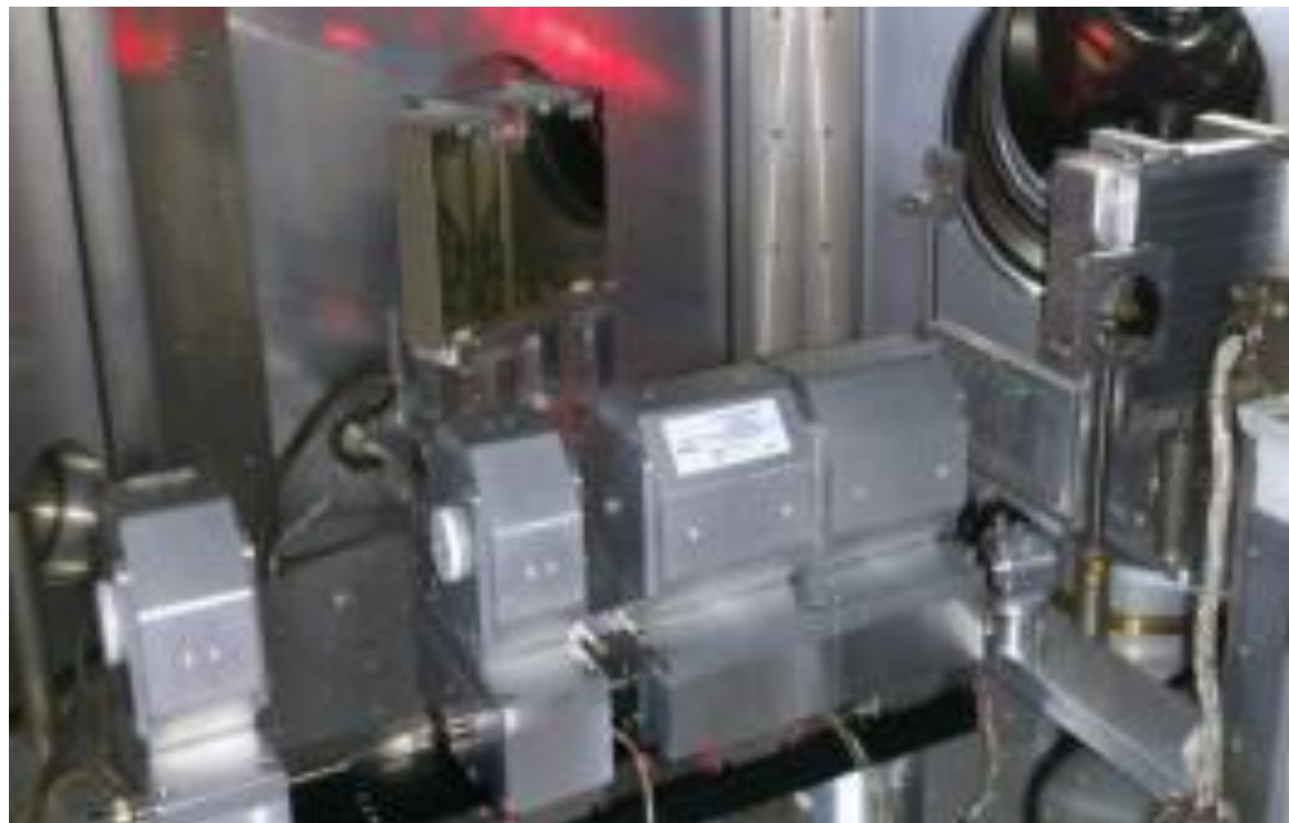
In vacuum Permanent Quadrupoles with displacement system for INFN ELI Gradient 100 T/m- Bore 36 mm
