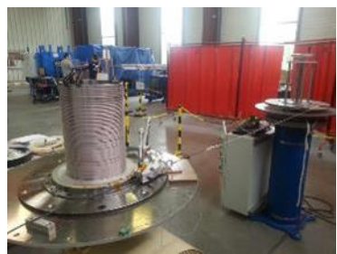
MgB2 coil tested at 460 A
