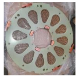
Fault current limiter coil
