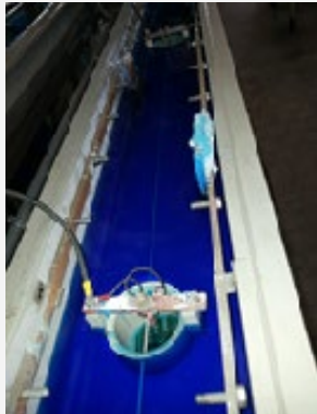
Ti-MgB 2 tape during copper plating
