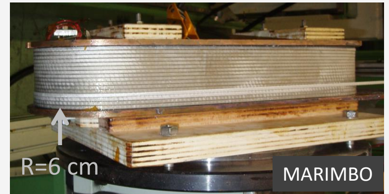
Winding of a racetrack coil with ex-situ MgB 2 tape
