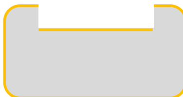
Groove machined by Turck head
