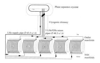
Thermosyphon Cooling Principle 1.5 kW @ 4.5 K refrigerator
