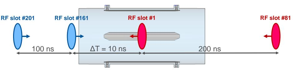
RF cogging by an RF expert: adjust ΔT from 10 ns to -10 ns in steps of ~ 1 ns, ~ 3 min / step (~ 1.5 hour)
