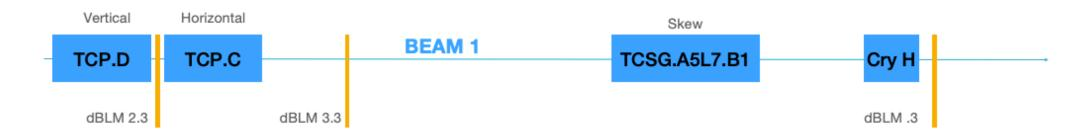
Part with single pilot bunches – Single Stage collimation hiearchy as used during commissioning – mask BIC Collimators/BLM
