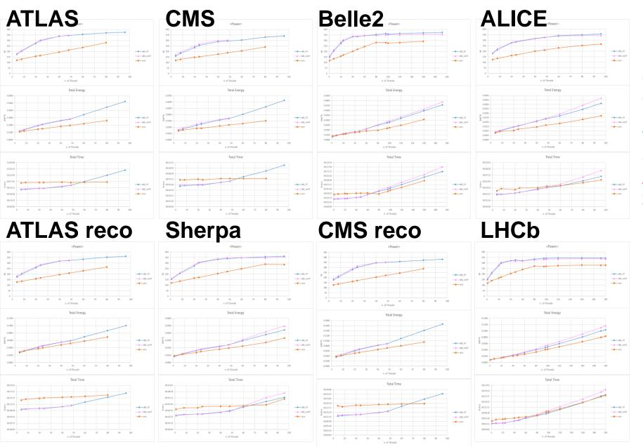
On **ARM**, the Energy (Power) increase linearly with the n. of threads, on **x86** saturates once hyper-threading starts.
