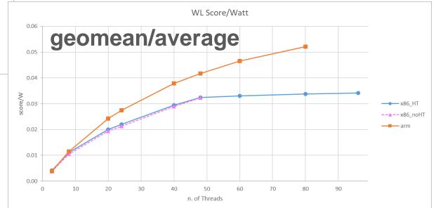
A physical x86 cores is faster than an ARM core, but rapidly lose the advantage once hyper-threading starts. ARM is always more energy efficient than x86 !
