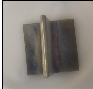
SS304 Plates With SS316L Filler Material Welding Corrosion
