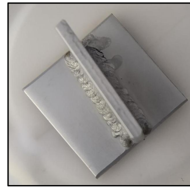
SS304 Plates With SS316L Filler Material Welding + Pickling & Passivation No corrosion
