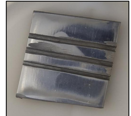
SS304 Plates With Machined Surface No corrosion
