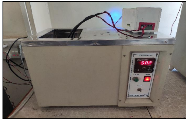
Setup: Water Bath Test temperature: 50°C Test Medium: Ultra Pure-water (1 sample) Gd loaded water (1 sample)
