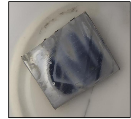
SS304 Plates With Machined Surface + Pickling & Passivation No corrosion
