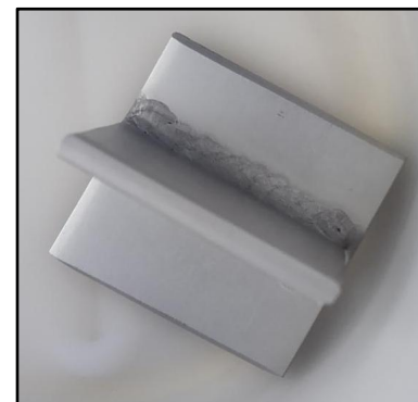
SS304 Plates With SS316L Filler Material Welding + Pickling & Passivation No corrosion
