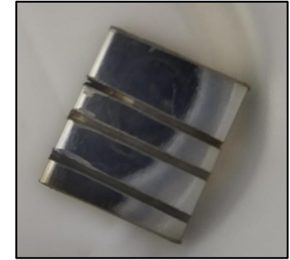
SS304 Plates With Machined Surface No corrosion
