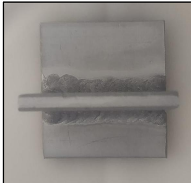
SS304 Plates With SS304L Filler Material Welding + Pickling & Passivation No corrosion
