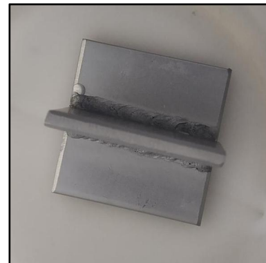
SS304 Plates With SS304L Filler Material Welding + Pickling & Passivation No corrosion
