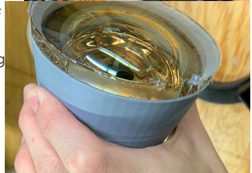
Gel damage during de-moulding - old jig
