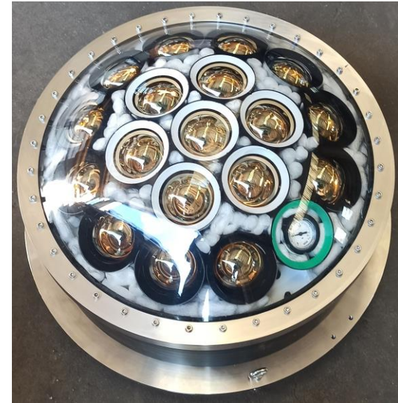
Prototype for the Implosion test, passed however
