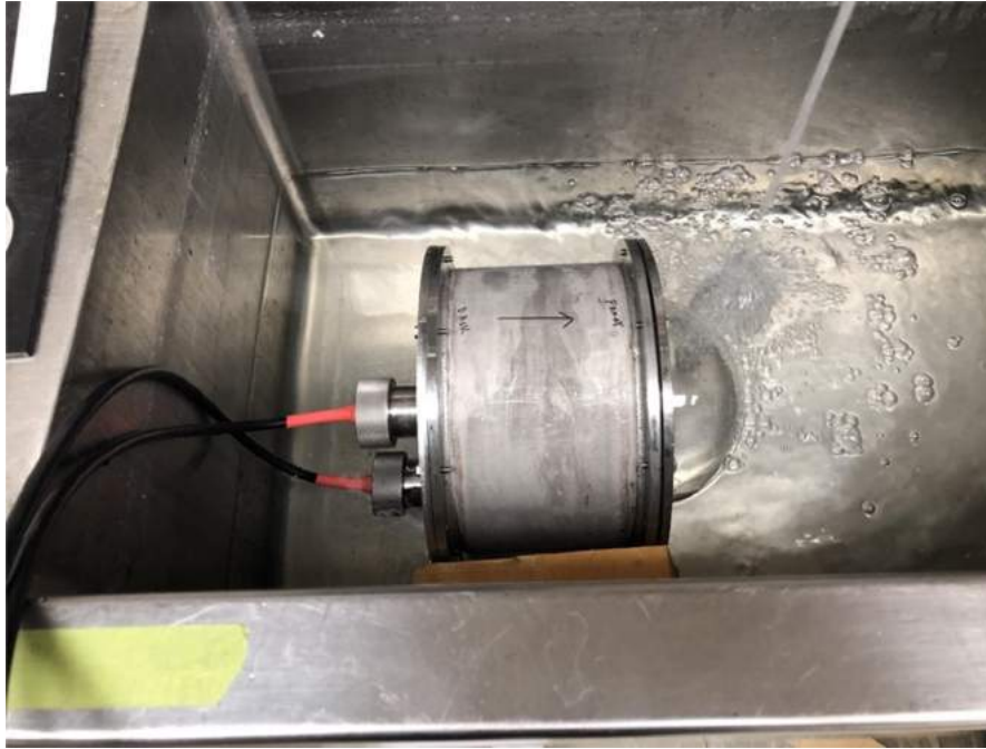
Test in sink had no leaks
