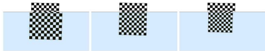
Fig. 3. Simulated Chessboard images with parts above and below the water line. The lens is misaligned forward (left), aligned (center), misaligned backwards (right).
