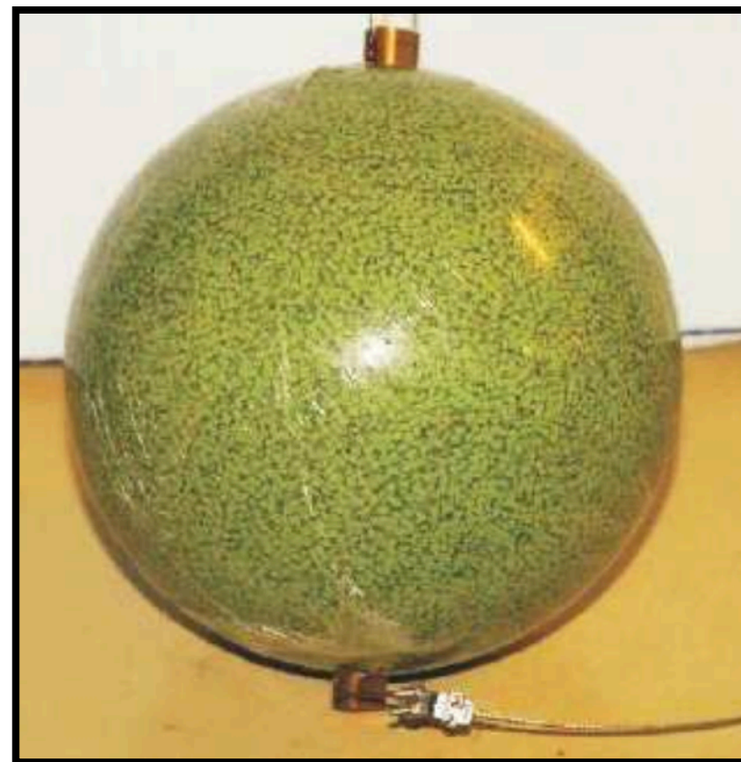
Nickel source used in SuperK ( https://arxiv.org/abs/1307.0162 )
