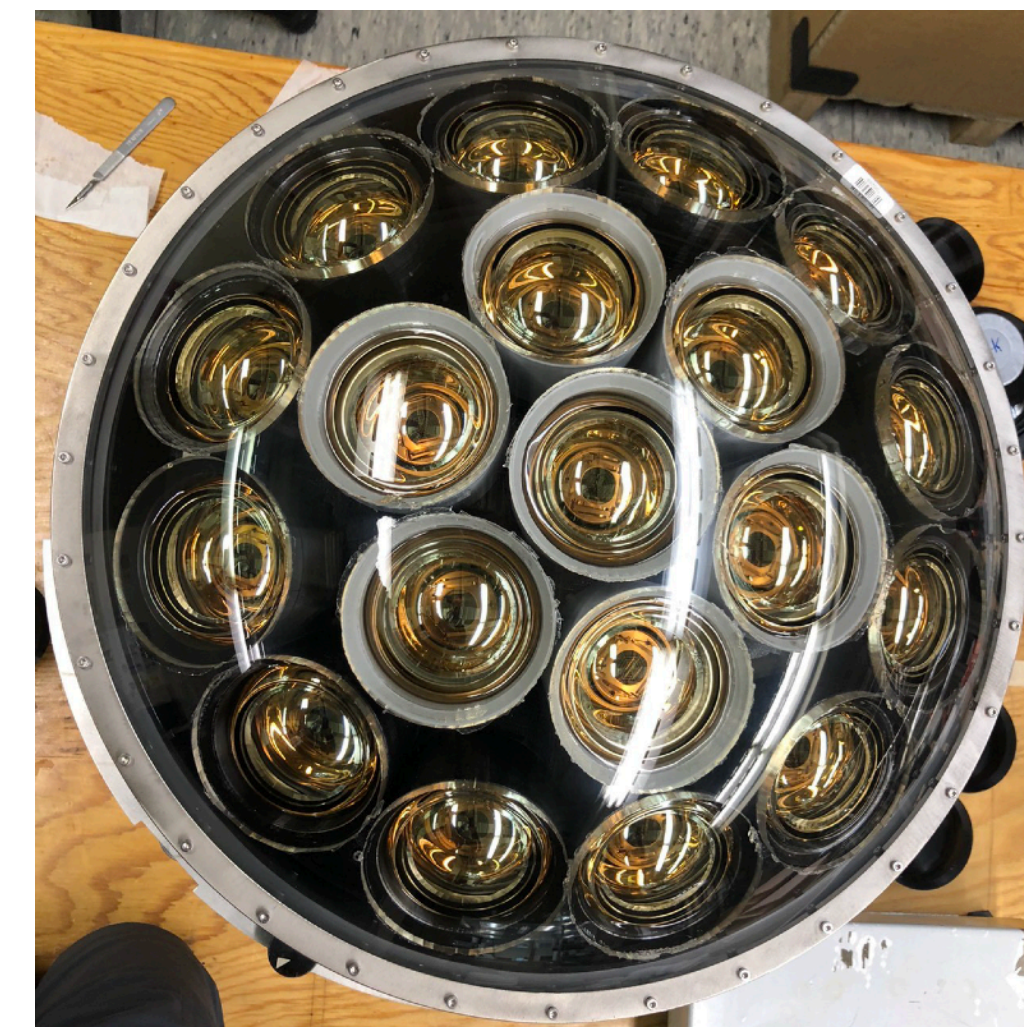
Ex-situ gel application prototype
