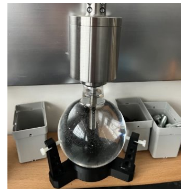
Prototype diffuser ball and preload mass (not yet filled with optical gel)
