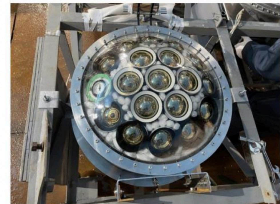
Installation in the mockup frame
