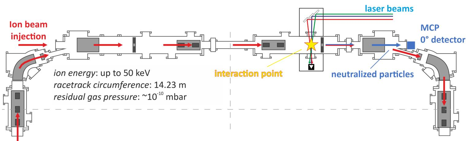
Optical grade vacuum windows have been installed at an interaction point of FLSR. The laser beam interacts transversally in this region of high ion density. The neutralized particles are detected downstream on a position sensitive detector.
