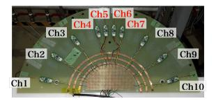
Figure 2: Prototype of multi-channel magnetic probes.
