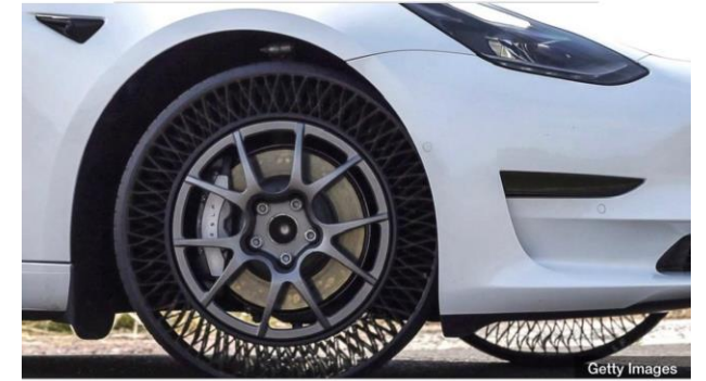
Plastic spokes support a thin tread on the Goodyear airless tyres
