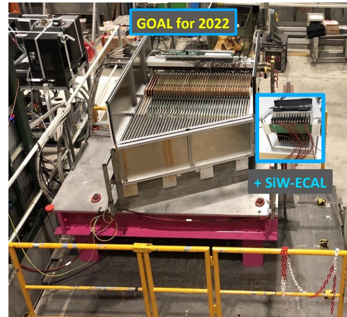
SiW-ECAL + AHCAL DAQ test @ DESY in March 2022
