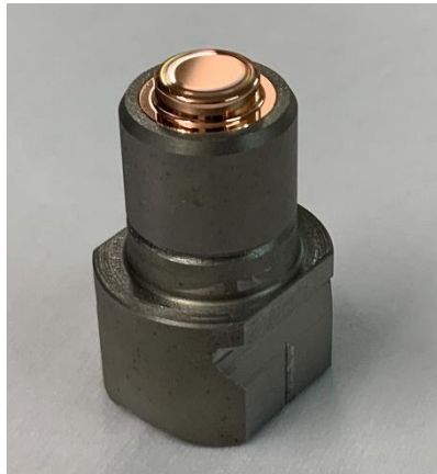
Hybrid Cu/Mo photocathode with off-centre diamond turned tip
