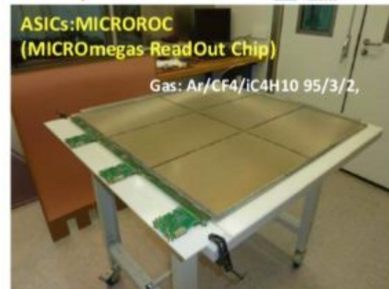
Micromegas prototype of 1x1m 2 consisting of six independent Micromegas boards
