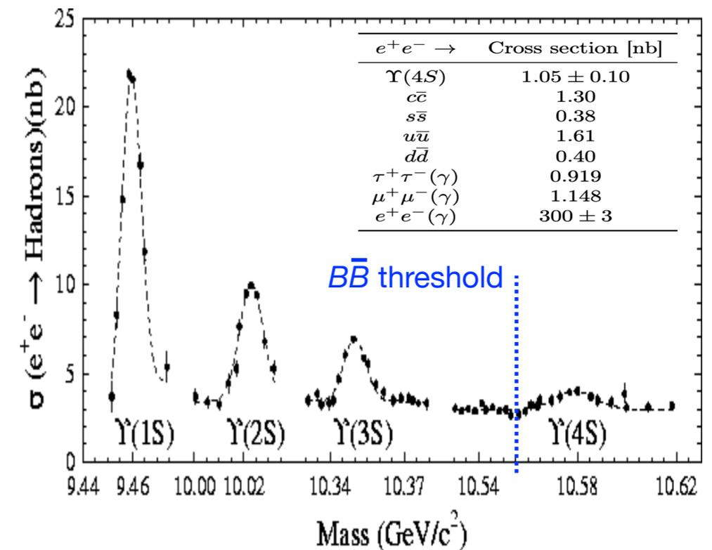
In B-Factories,  $e^+$  and  $e^-$  collide at 10.58 GeV to make  $\Upsilon(4S)$  resonance decaying into  $B^+B^-$  and  $B^0\bar{B}^0$  in 96% of the time. Belle ( $\sim 1 \text{ ab}^{-1}$ ) and BaBar ( $\sim 0.5 \text{ ab}^{-1}$ ) played a crucial role in establishing large **CP violation** in the B-meson system in the SM and constrained on the **CKM matrix**.
