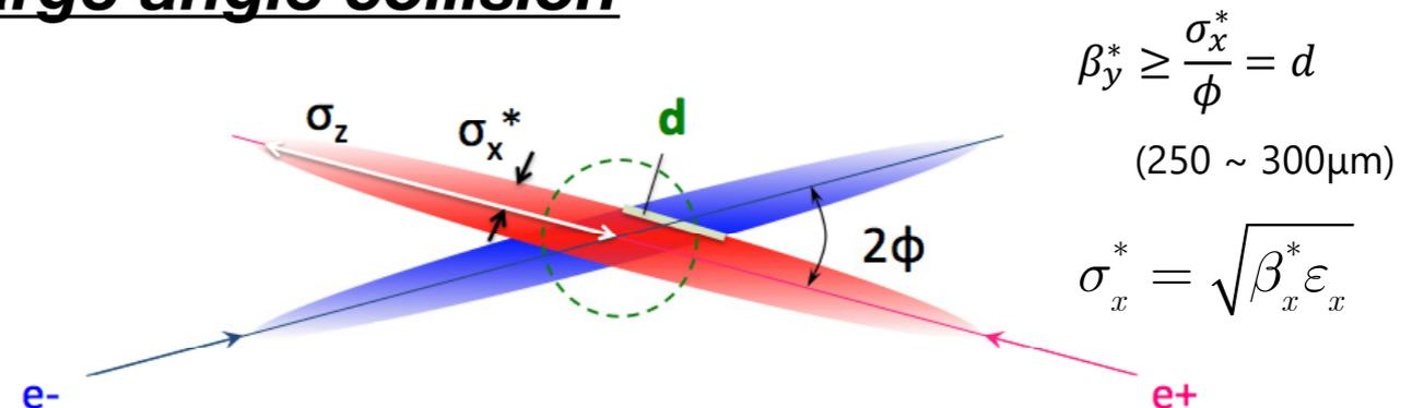
Due to hourglass effect, the luminosity does not increase when  $\beta_y^* < \sigma_z$ .
