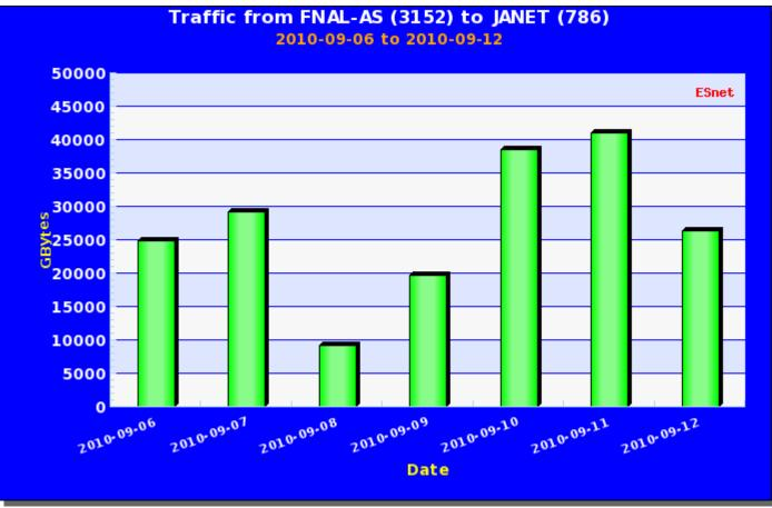
Recalling that moving 10 TBy in 24 hours requires a data throughput of about 1 Gbps, the graph above implies 2.5 to 4+ Gbps of data throughput – which is what was being observed at the peering point
