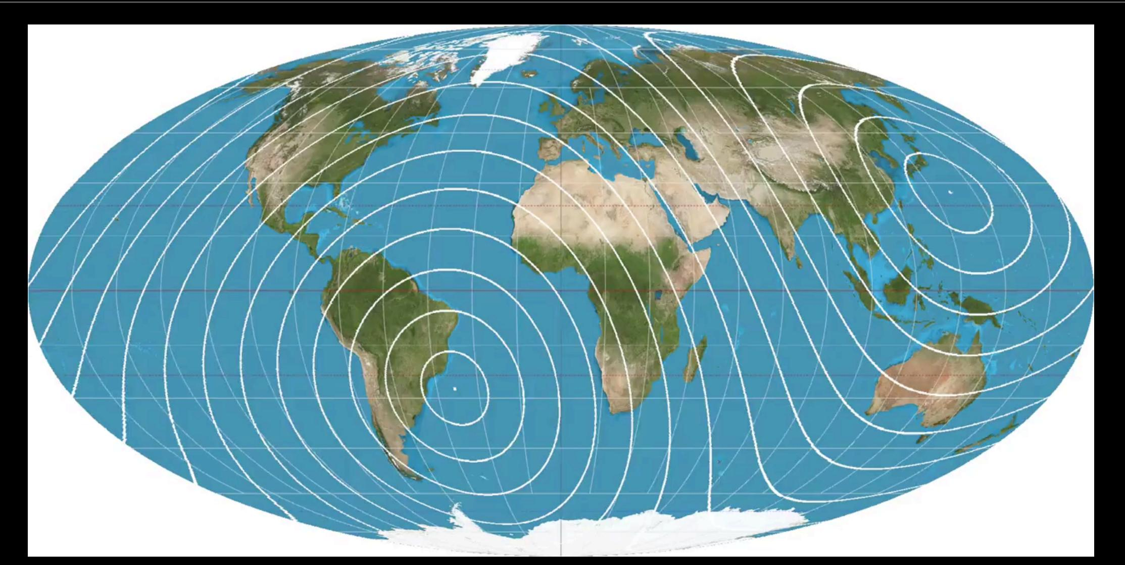
The white circles indicate positions in the sky map that will have equal time/phase delay when the signal from that part of the sky arrives in the LIGO Hanford and Livingston detectors.
