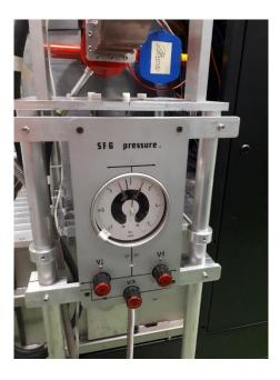
Used with SF6 for RF photo injectors in CLEAR and AWAKE at CERN, the DEFT machine at CHUV will need one as well. Many more circulators are used at CERN of course, but not filled with SF6 due to lower peak power
