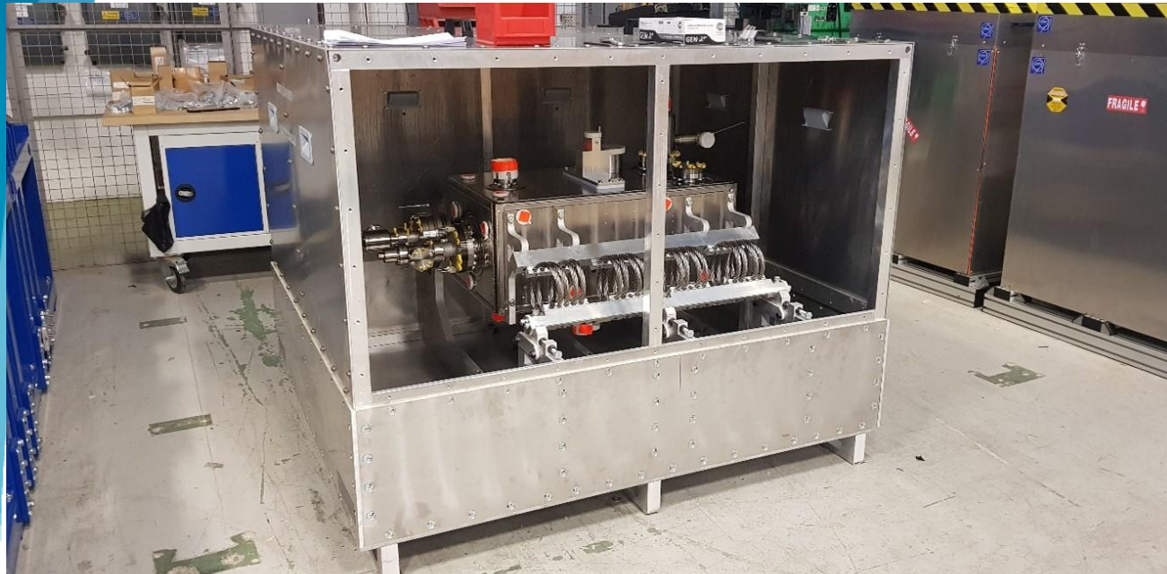
RFD Cavity in Transport Frame on arrival at Daresbury Laboratory
