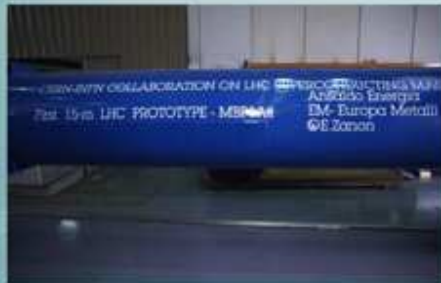
First prototype of 15 m superconducting LHC dipole by CERN-INFN-Ansaldo Energia collaboration, 1998.
