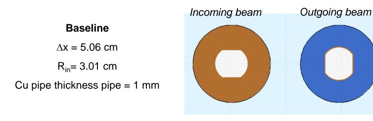
Larger aperture to mimic mechanical/alignment tolerances
