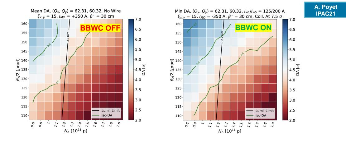
Simulations (and B2 observations in the 2018 MD) show that it will be difficult to gain more than ~10 µrad in the crossing angle at the EoL in Run3 (we focused on the 2022 Run).
