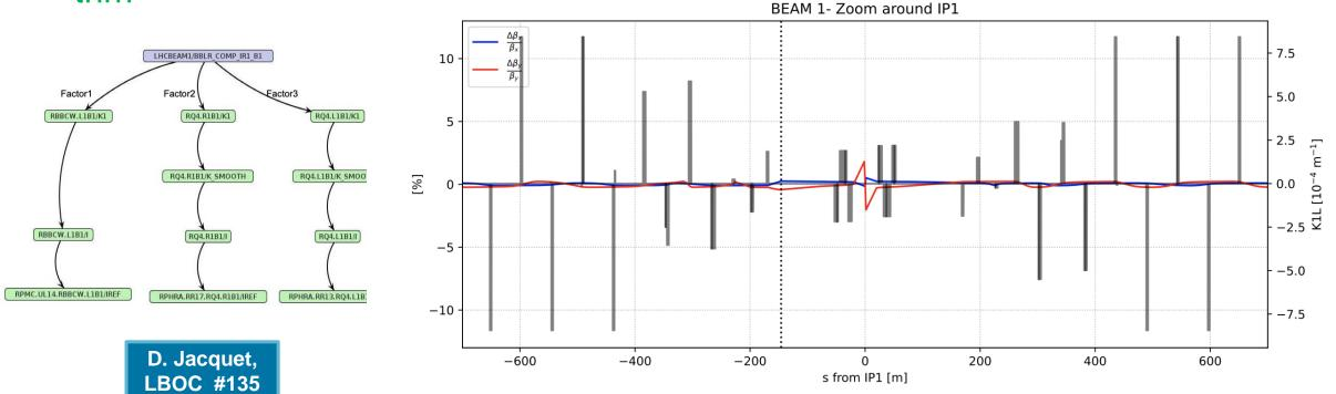
Using the Q4L/R correct the tune but not (fully) the induced beta-beating:  $\rightarrow$  minor effect on luminosity (<0.1%)
