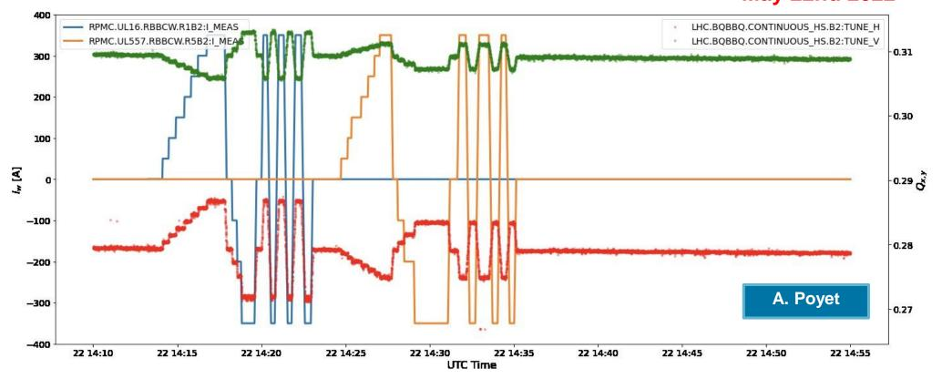
All 4-wire polarities were checked successful with beam at injection (B2 shown in the picture).
