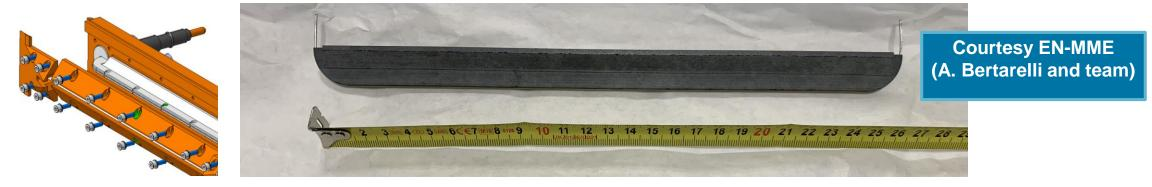
Results (out/in vacuum) are not yet circulated (EDMS 2432228): the tests were done with 1 mm and 0.8 mm radius molybdenum wires.
