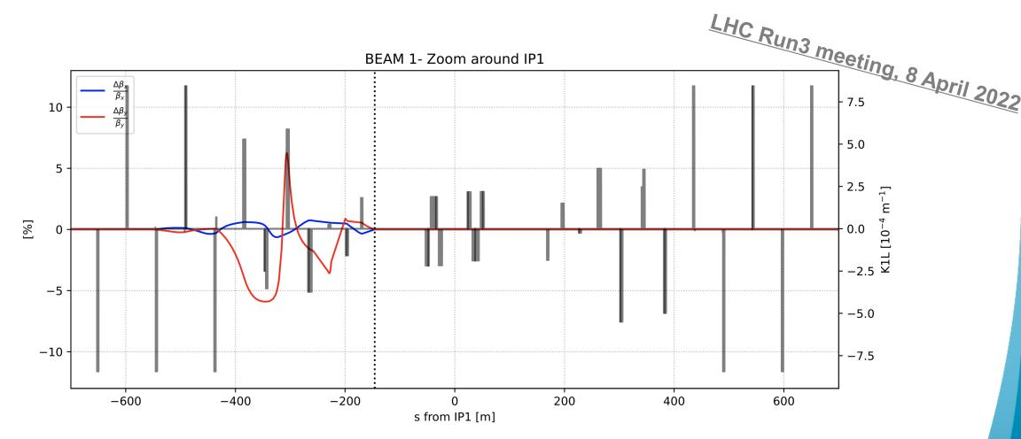
A Q13-Q4 correction was studied (Q6-7 not included) to rematch properly the IP optics. → Solution is available and can be tested during MD in 2022 and deployed later stage
